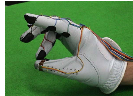
Universal Keyboard Using Chording Gloves [ http://iesys.skku.ac.kr/~human/ ]
